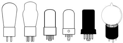
The picture above shows common bulb styles. From left to right they are: S-bulb (also called globe or balloon); ST-bulb (also called shouldered or "G" style); T-bulb (tubular, if an 8 pin base referred to as "GT "or "GT/G"); T-bulb with a Loktal base; MT-bulb = metal tube; G-bulb (also called ball or tennis ball).
